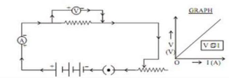
Ohm's Law  $\rightarrow$ He stated that the electric current flowing through a conductor is directly proportional to the potential difference across its ends, under standard temperature and pressure conditions.  $V \propto I$
